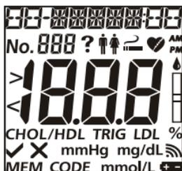
After startup, the Initial Screen will be displayed. Ensure the code chip is inserted. Compare the number showed in the display with the code number printed on the canister label or foil pouch. Refer to Initial Setup. The **test device symbol** will flash when the meter is ready for the device to be inserted.
