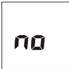
If the meter displays ***no***, check the control device for contamination or to check if it is damaged. If there are any visible signs of damage or contamination, discard the control device and retest using a new device.
